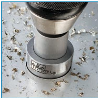
**Quickly drills precise holes without penetration beyond sheet metal.**
