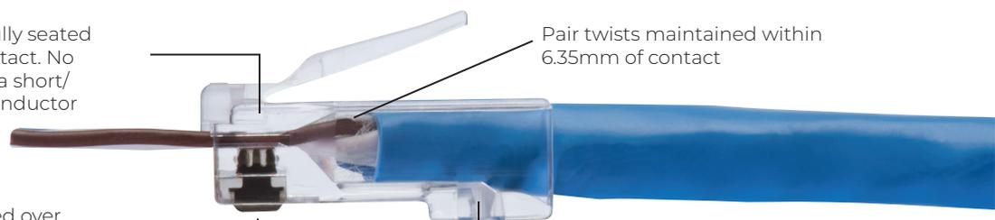
Pair twists maintained within 6.35mm of contact
