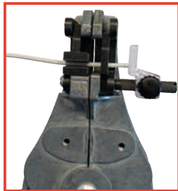
Transparent wire stop provides uniform stripping length
