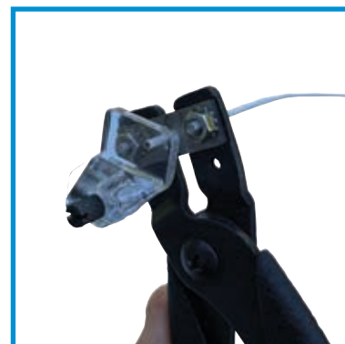
Adjustable wire stop for precision strip lengths
