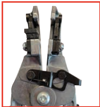
Short-stop latch protects wire strands by limiting the stripping stroke to 4 mm (5/32") and retains the slug until the wire is ready for termination
