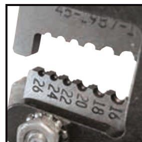
High precision counter-bored die type blades
