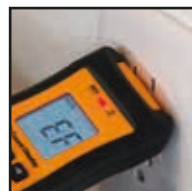
NCVT in tip detects presence of AC voltage
