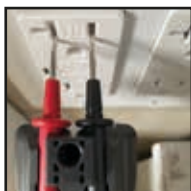
Probe Holders are spaced to test tamper resistant outlets
